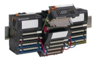
Electronics can be replaced without detaching wiring. So there is no additional work for rewiring and minimized costs through reduced stoppage times. Mechanical coding prevents insertion of incorrect electronics.
